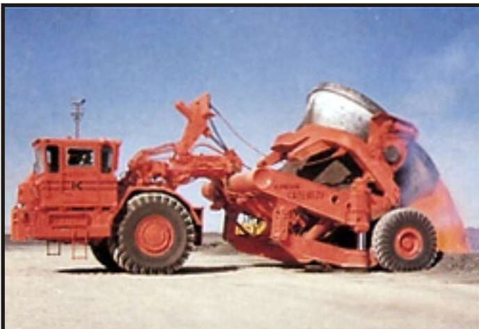
Kress "P-E" Series slag pot carriers, featuring the use of small earthmover rear tires, are available in capacities for 35 tons (32 tonnes) to 120 tons (109 tonnes).
