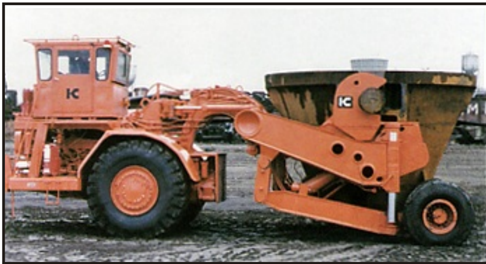
Kress "P" Series slag pot carriers are available in capacities from 35 tons (32 tonnes) to 210 tons (190 tonnes).
