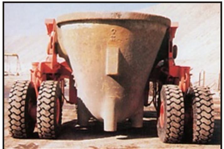
Kress "P-E" Series slag pot carriers, featuring the use of small earthmover rear tires, are available in capacities for 35 tons (32 tonnes) to 120 tons (109 tonnes).
